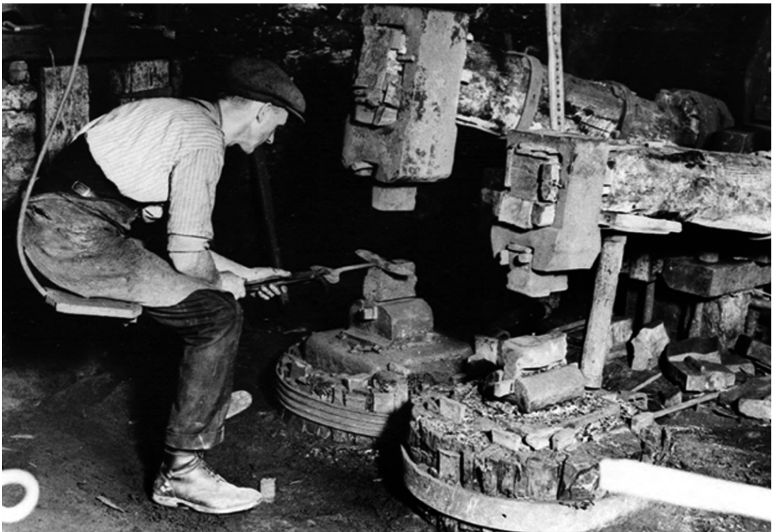
FIGURE 4: Pair of tilt hammers at Holbeam Mill, Devon, c.1930.
